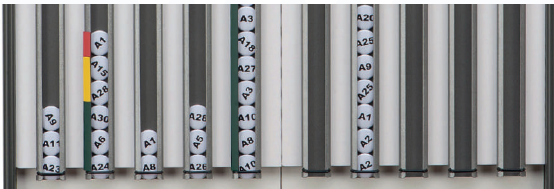
Fig. Detail FiFo row equipped with coins and magnetic strips in traffic light colours – the solution in the small-parts or pallet warehouse.
